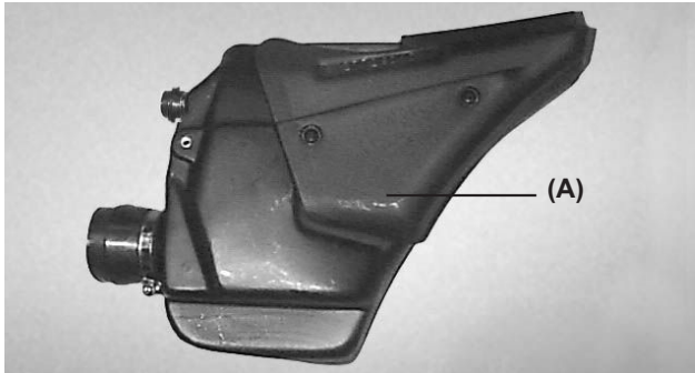
(A). Air filter box.
